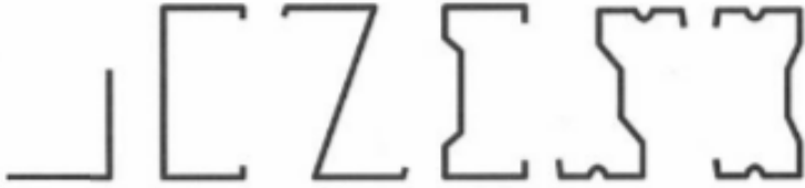
Figure (1.5) Cold-Formed Long Products (Examples of Sections T and S)
