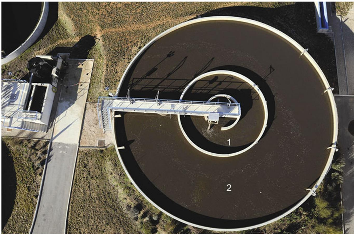
Figure 18 : Aerobic treatment tank. 1 Anaerobic zone, 2 aerobic and anoxic zone
