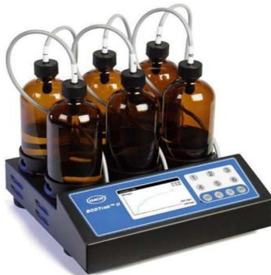
Figure 8 : Measuring apparatus for BOD
