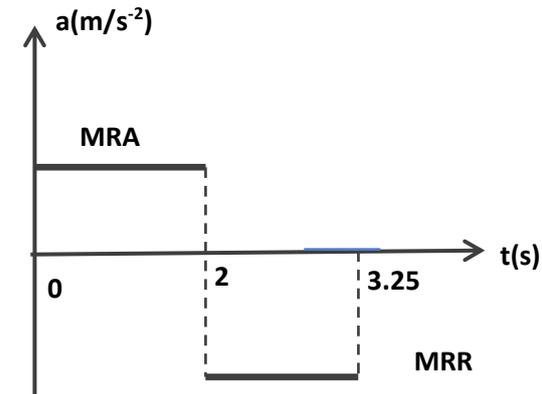
$$t \in [0, 2]s, a_1 = \frac{\Delta v_1}{\Delta t} = \frac{4-0}{2-0} = 2 \text{ m} \cdot \text{s}^{-2},$$
