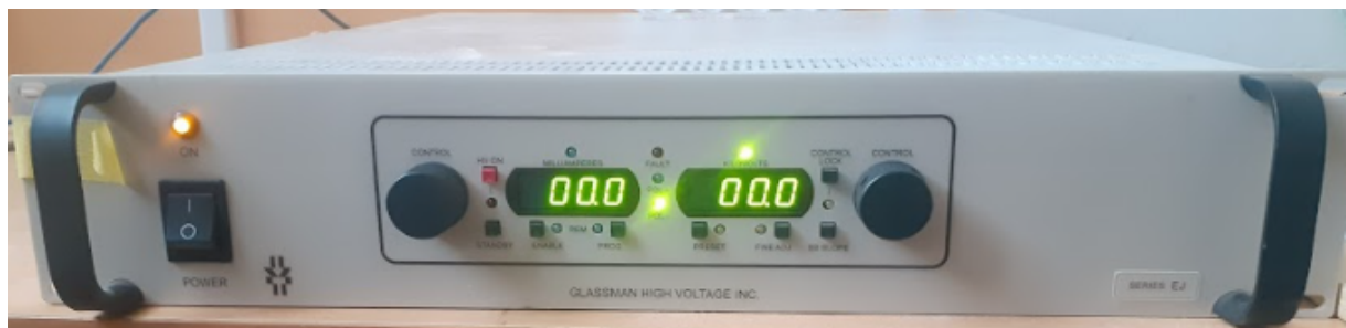
Figure III. 2: Source haute tension continu (XP Glassman, 40 kV, 15 mA).
