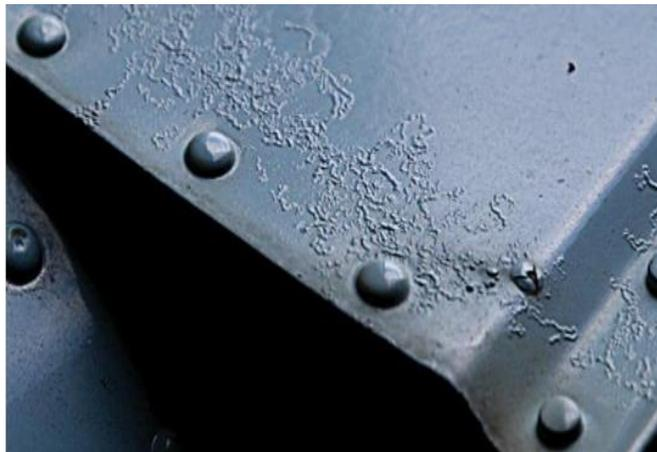
Figure I.14 : corrosion filiforme [18]
